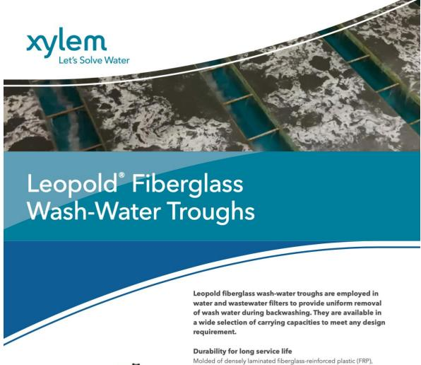
Molded of densely laminated fiberglass-reinforced plastic (FRP), Leopold wash-water troughs are corrosion-resistant and constructed for maintenance-free durability and long service life. All mounting brackets, hardware, and stabilizers are stainless steel.
